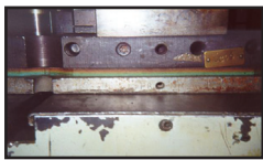
Thermal degradation of insulator board
