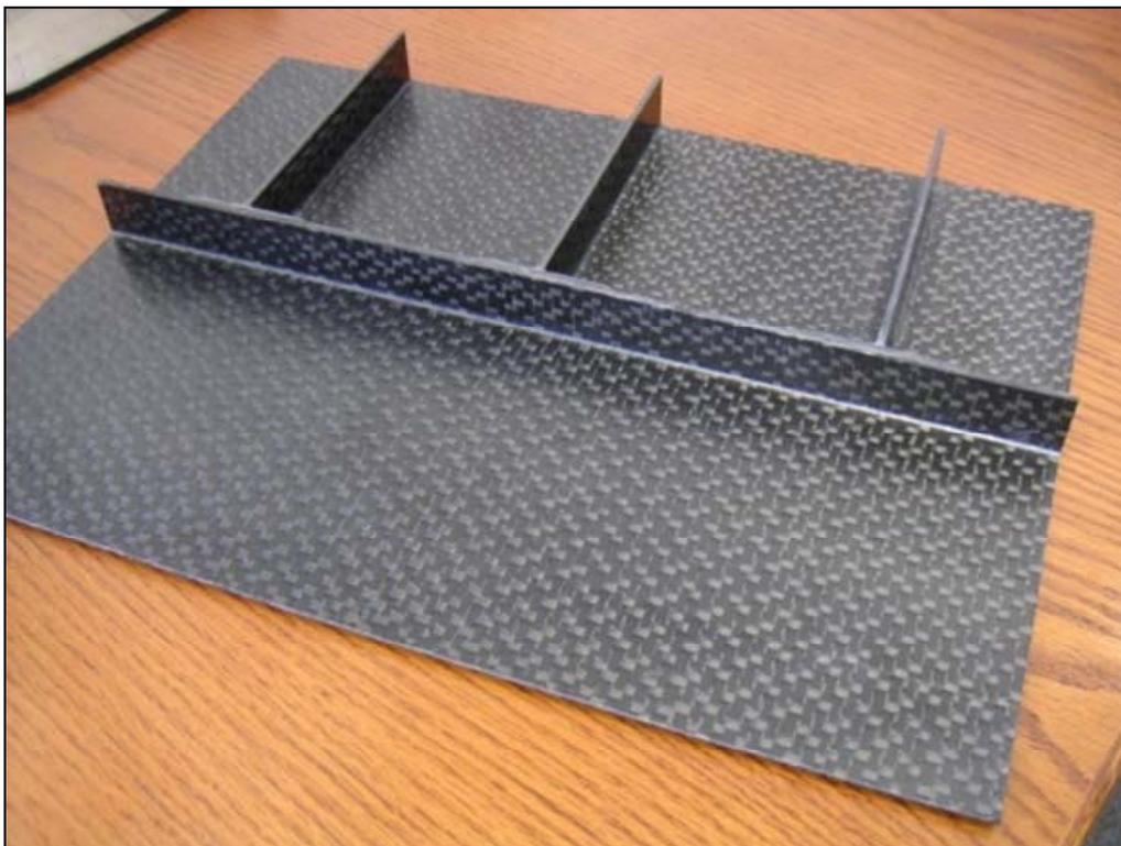
Figure 2 – Stiffened panel utilizing a 3D woven fiber preform
