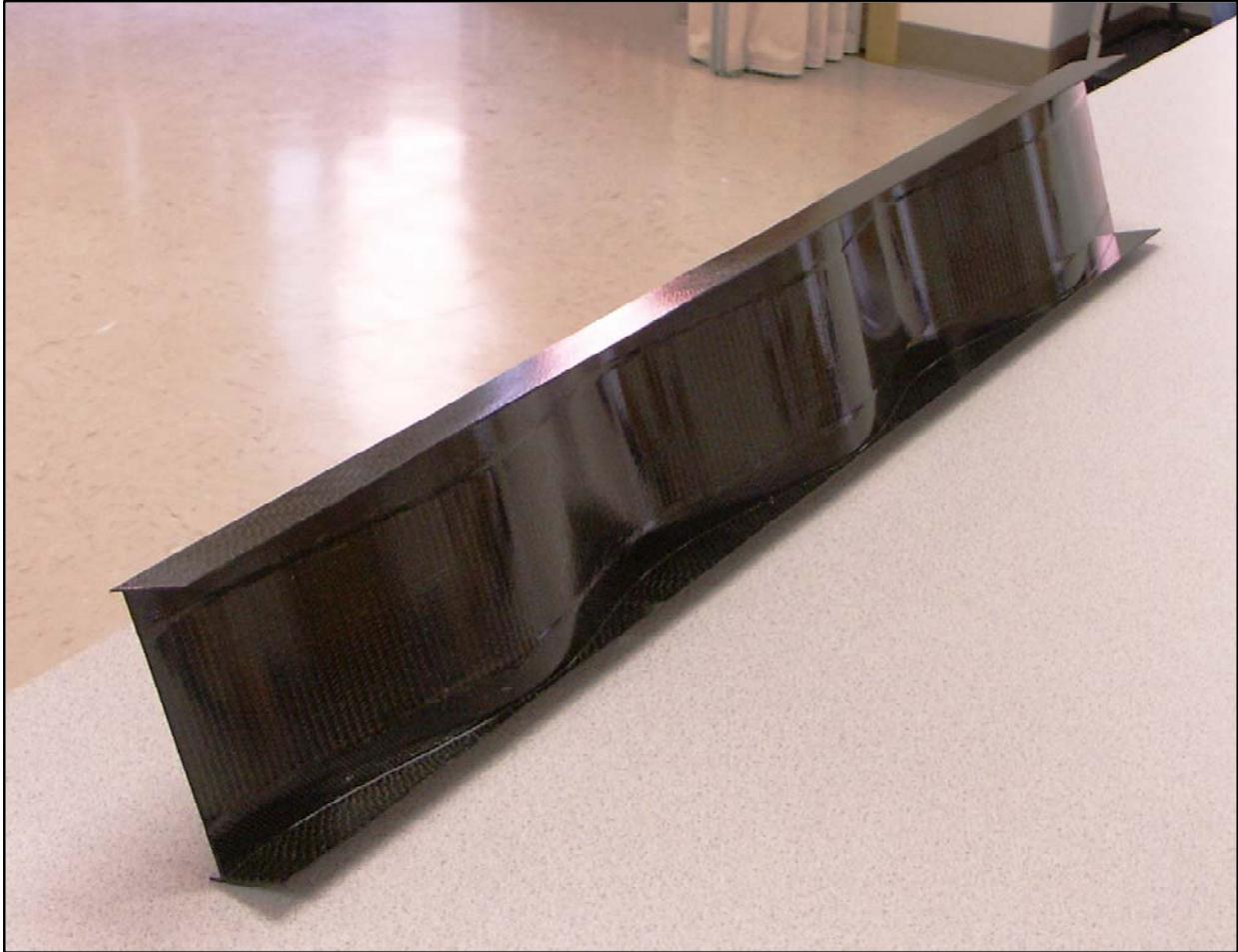
Figure 4 – Prototype sine wave web beam
