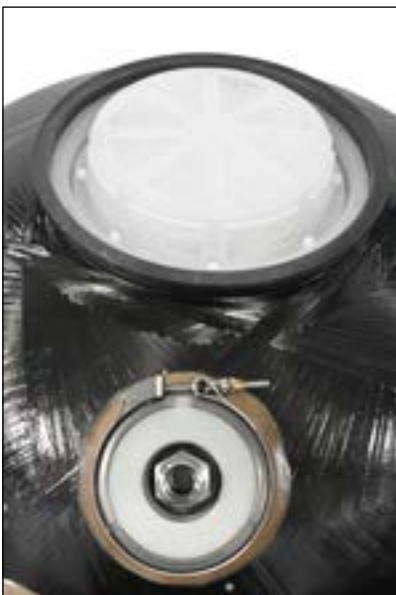
Filter Canister Assembly Installed
