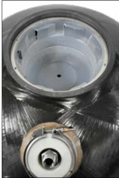
Outer Bowl & Shroud Installed
